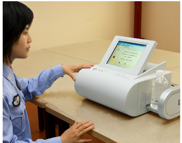
A water bottle is tested with the AY01-01 Rapid Liquid Contraband Detector, enabled by Ocean Optics' QE65000.
