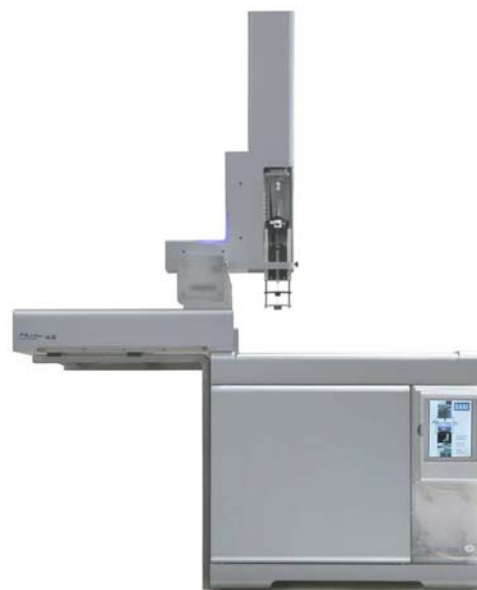
MASTER GC Fast Gas Chromatograph equipped with MASTER AS Liquid Autosampler.
